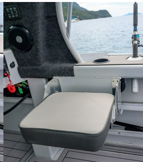
This dickey seat is a useful step up when getting on or off the boat. When not in use it folds unobtrusively away.
