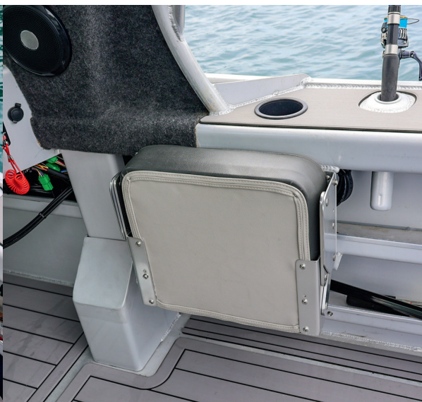
This dickey seat is a useful step up when getting on or off the boat. When not in use it folds unobtrusively away.
