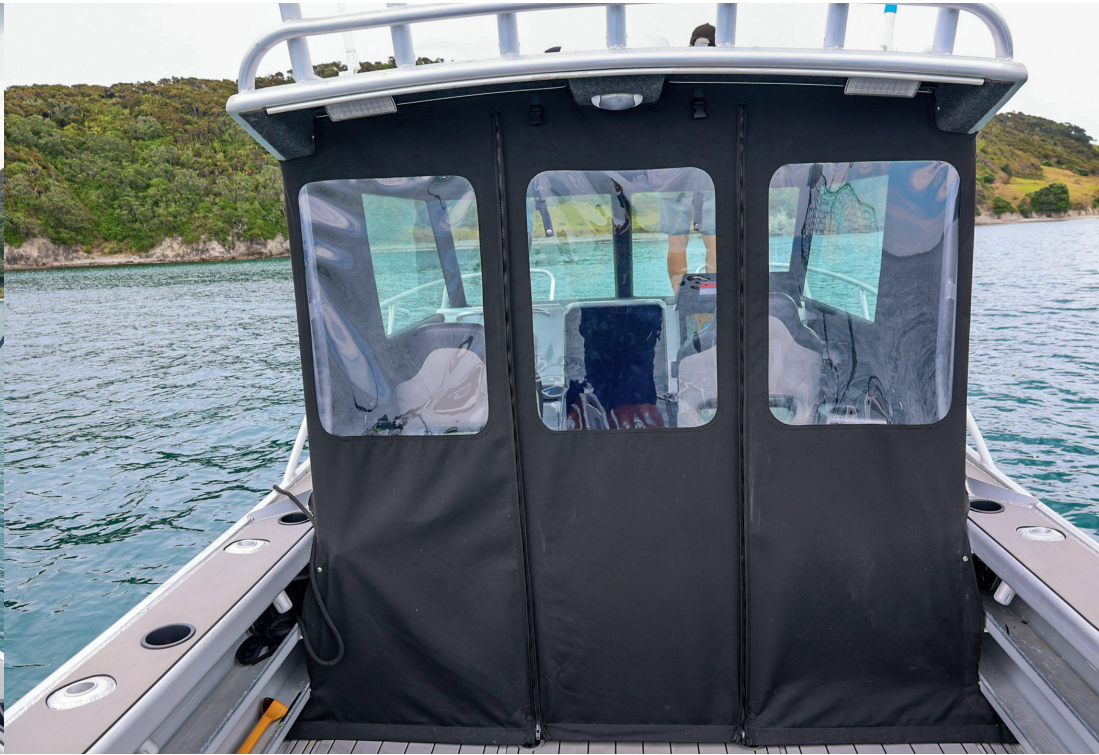
The cockpit space is increased with the removal of the cockpit dropdown curtains, which provide protection in adverse conditions or when overnighting.
