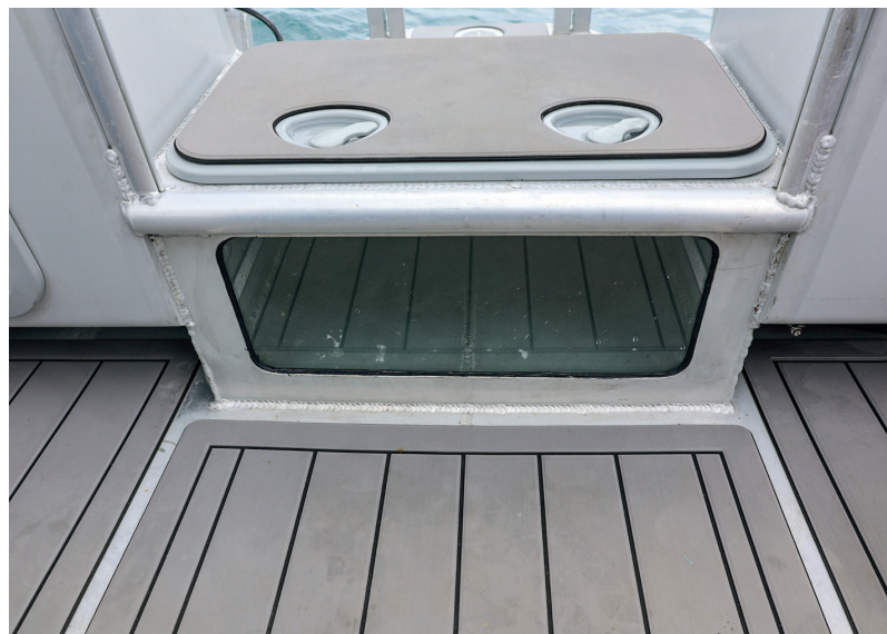
Set into the step through to the rear platform is the livebait tank. Right: This baitboard can be placed on either side of the transom.
