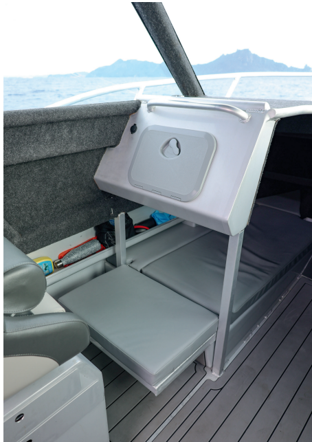
From left: A Softrider pedestal takes some of the bumps out of the ride for the helmsman; The saltwater sink is ideal for washing bloody or slimy hands; When overnighting, extra length is added to two berths thanks to the folding upholstered footrests.
