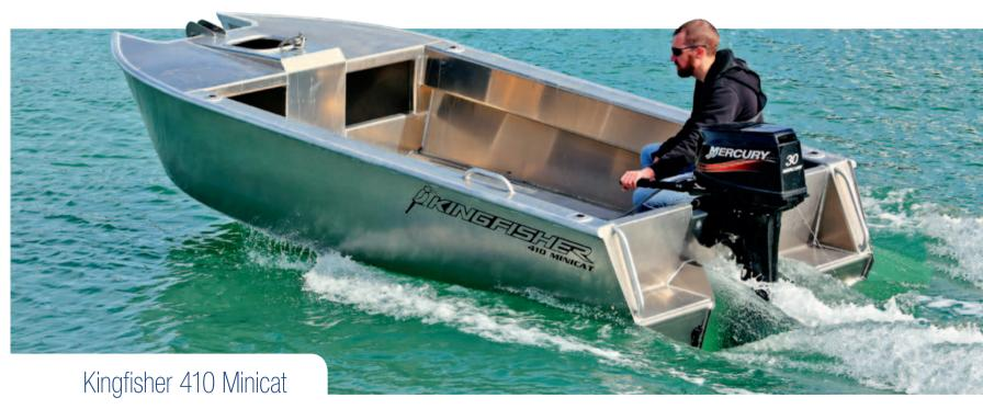
**LONGER, BEAMIER AND** heavier than the 370, the 410 is also a fairly basic package, but offers more internal volume. Built from 3mm and 4mm aluminium with 4mm tread-plate floor, it's designed for a single outboard of between 20hp and 40hp.
