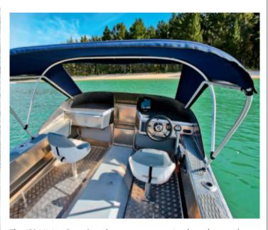
The 450 Minicat Front Steer has a more conventional, runabout-style layout with a split dodger opening onto the foredeck. The raised wingdeck could be used to advantage for fixing a chilly bin or other removable storage. There's good access to the transom and sides, and like the rest of the range, stability is impressive.
