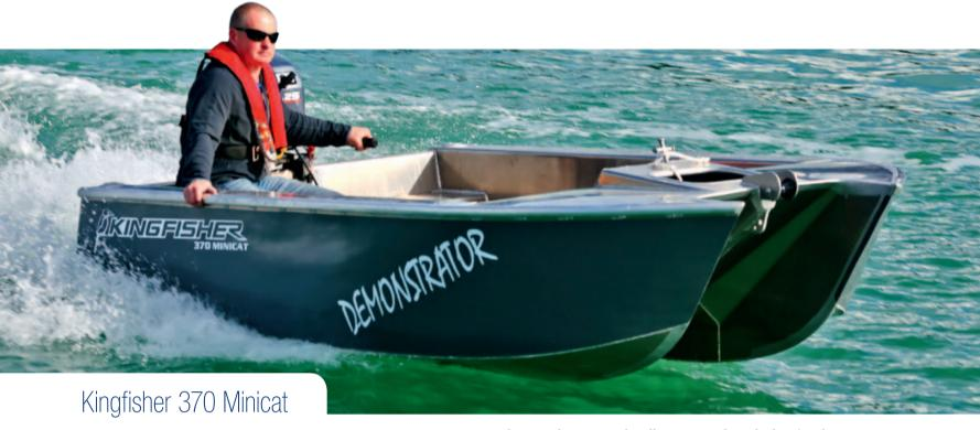
**WITH A HULL** weight of only 200kg, this 3.7m open dinghy provides an amazing amount of internal space and is easily driven by outboards in the 15 to 30hp range. Designed for inshore boating, it's the spiritual successor to the old 12-foot tinnie, but strongly built in 3mm aluminium with a 4mm tread-plate floor.
